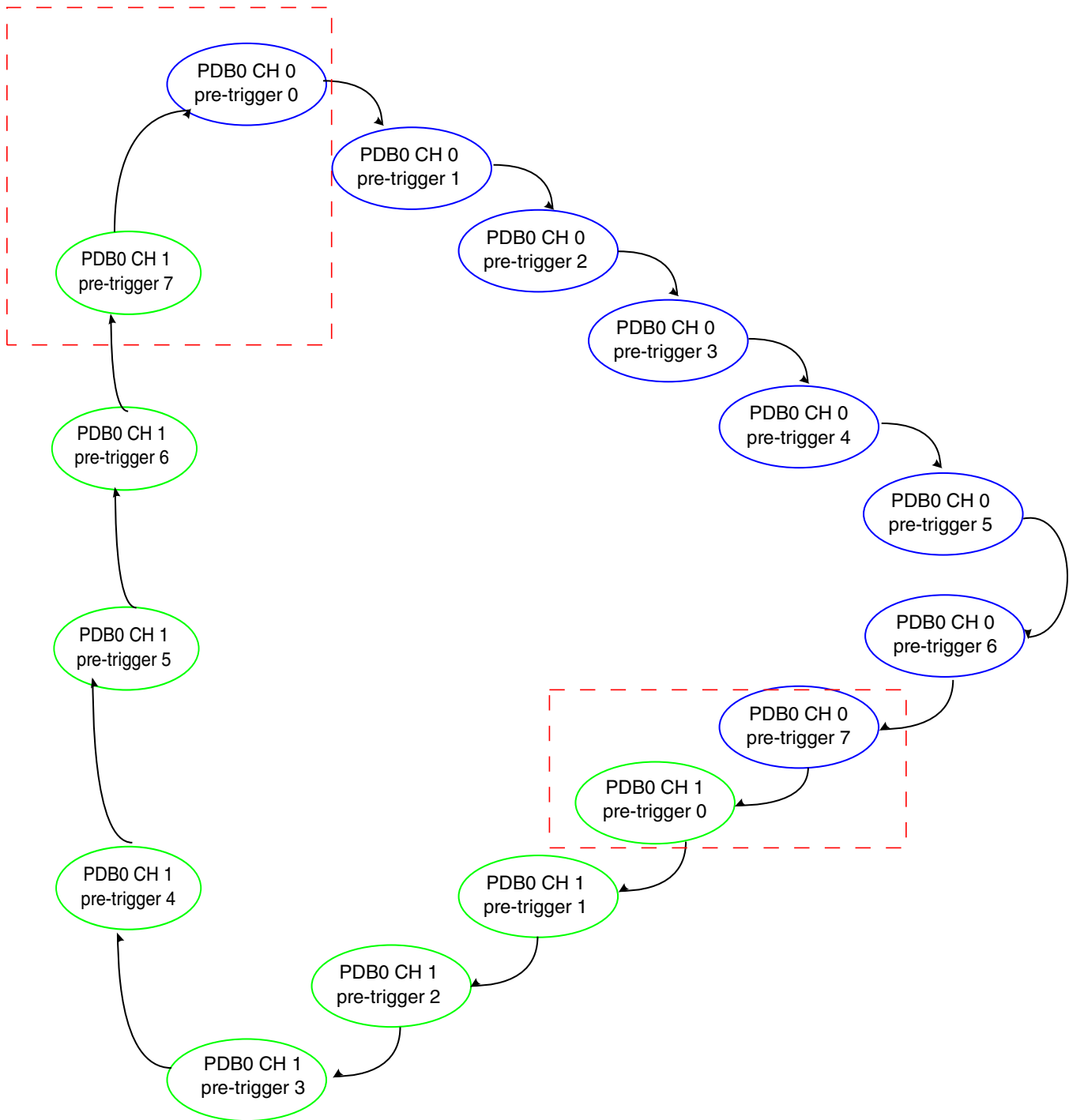
Figure 46-4. PDB back-to-back chain forming PDB0-PDB1 ring
